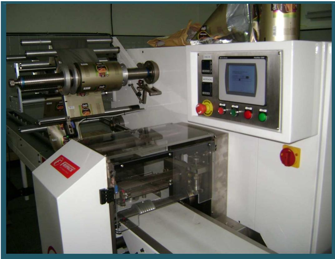
Figura 3.14 Máquina envasadora Flow-pack
